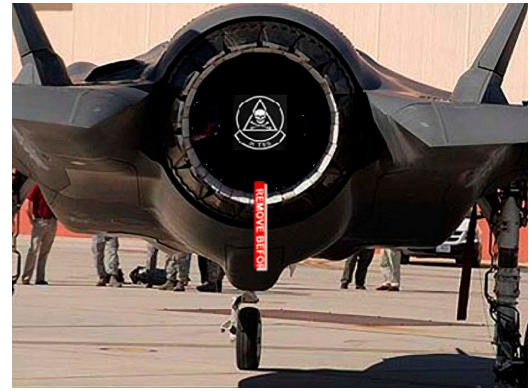
Joint Strike Fighter F-35 Exhaust Plug
