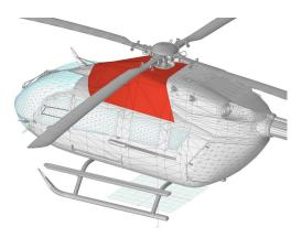
Barrier Inlet Filter Cover, 3D Rendering
