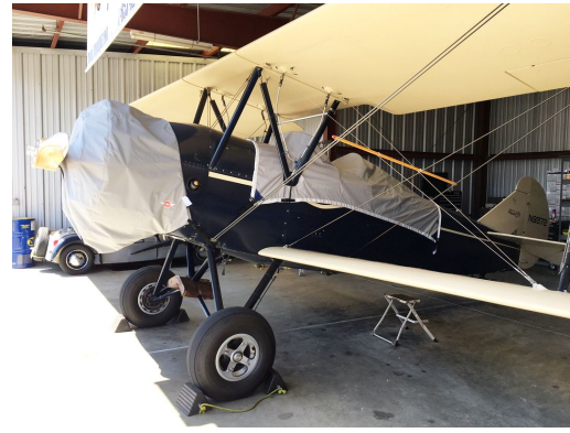
Travel Air 4000 Canopy and Engine Covers, light weight travel type
