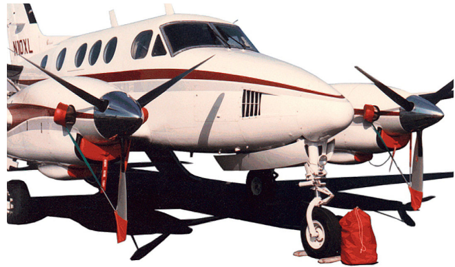
Pitot, Exhaust Covers, Engine Plugs & Prop Ties
