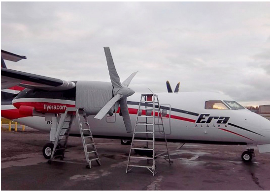
Dash 8 Insulated Engine & Prop Covers
