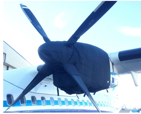
ATR-72-202 Insulated Engine & Prop Hub Covers
