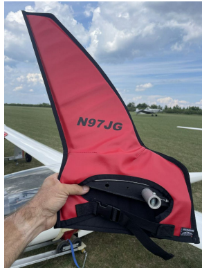
Schempp-Hirth Ventus-2B winglet/wingtip pads
