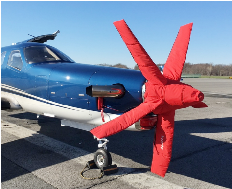
Socata TBM Insulated 5-Blade Prop/Spinner Cover Pilatus PC-12 Exhaust Cover, Fully Enclosed, for protection against corrosion.
