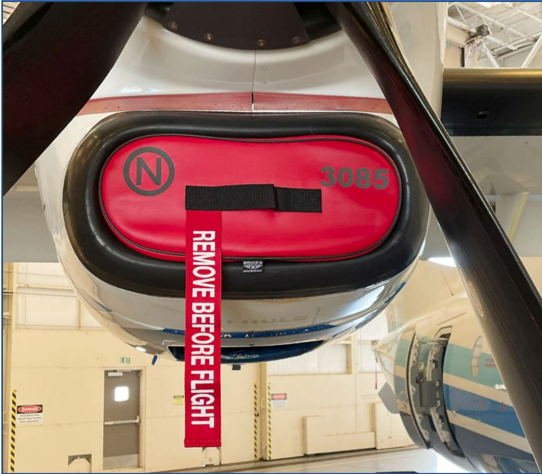
Dornier 328 Turboprop Engine Inlet Plugs
