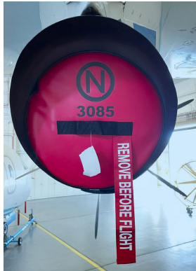
Dornier 328 Turboprop Engine Exhaust Plugs
