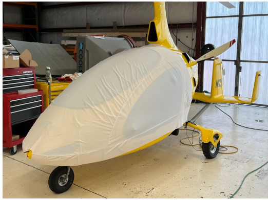
Autogyro Cavalon Canopy/Nose Cover, test fit cover
