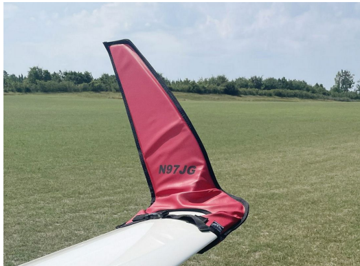
Schempp-Hirth Ventus-2B winglet/wingtip pads
