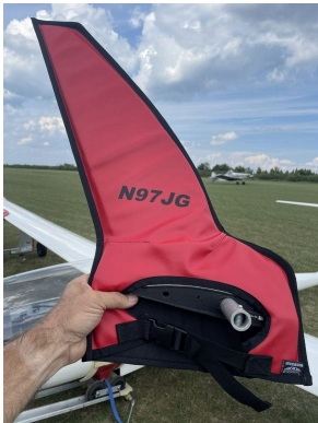
Schempp-Hirth Ventus-2B winglet/wingtip pads
