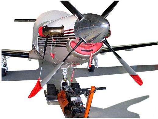
Pilatus PC-12 LARGE ENGINE INLET PLUG, SMALL PLUGS SET, Prop Tie/Exhaust Covers
