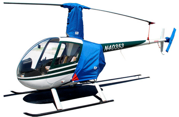
Robinson R-22 Engine, Rotor Mast & Tail Rotor Covers, with Blade Tie-down
