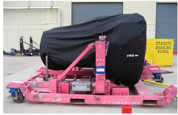
CFM-56-7 Off-link Engine Long-term Storage "Rain Cap" cover, w/o Exhaust Cone, fully enclosed
