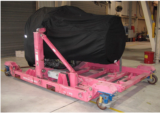
CFM-56-7 Off-link Engine Long-term Storage "Rain Cap" cover, w/o Exhaust Cone, fully enclosed
