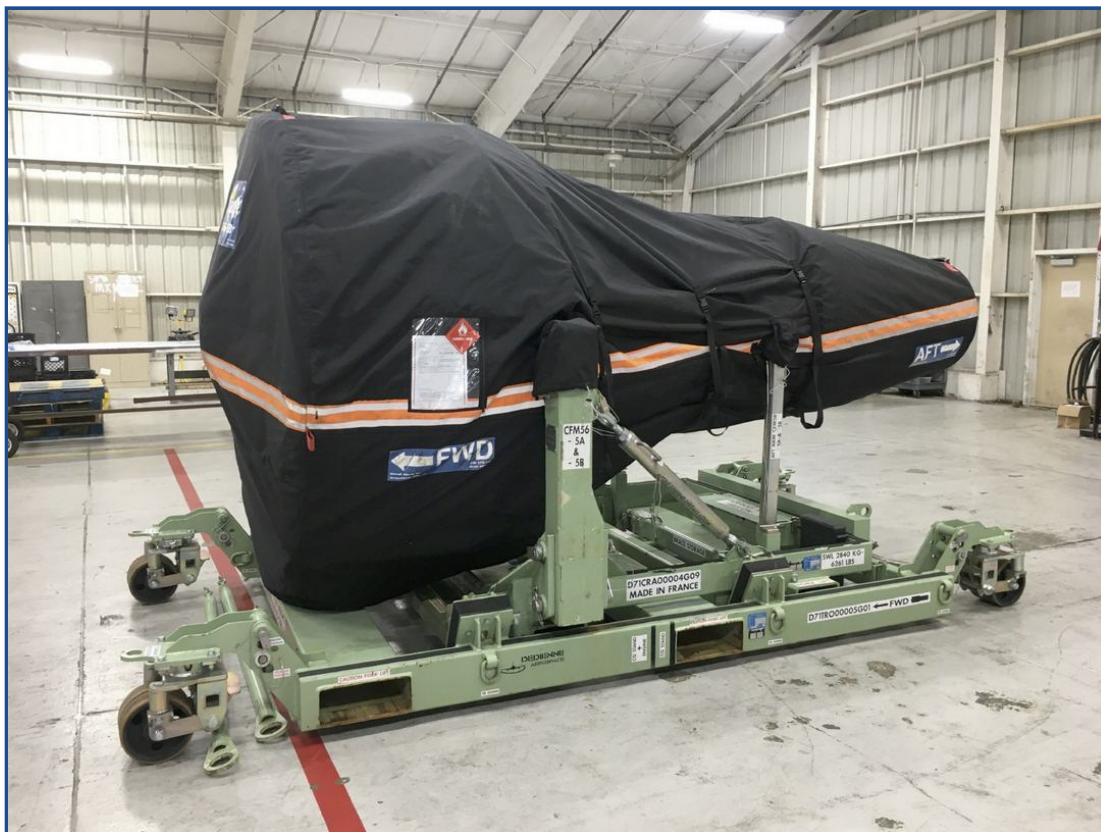
CFM56-5B Off Link Cover, fully enclosed
