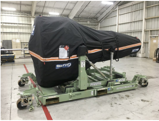
CFM56-5B Off Link Cover, fully enclosed
