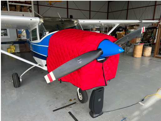
Insulated Hangar Blanket on Cessna 182
