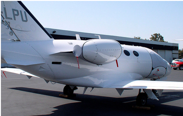
Citation Mustang Light Weight Engine Cover, Light Weight Windshield Cover, Pitot/AOA Cover
