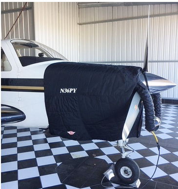
Beech Bonanza 36 Models Insulated Engine Cover
