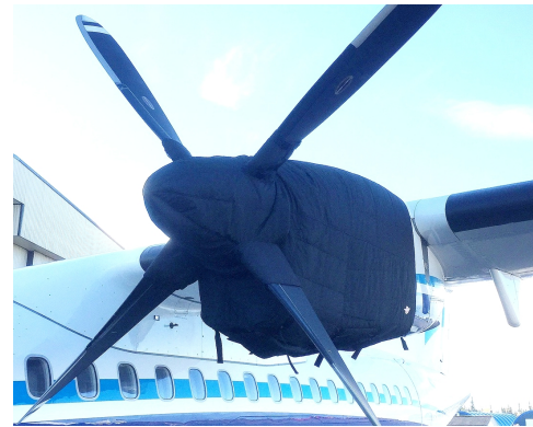
ATR-72-202 Insulated Engine & Prop Hub Covers
