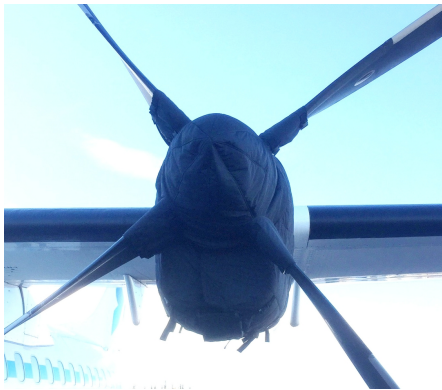
ATR-72-202 Insulated Engine & Prop Hub Covers
