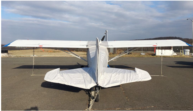
Maule M-5-235C Extended Canopy Cover, Empennage Cover
