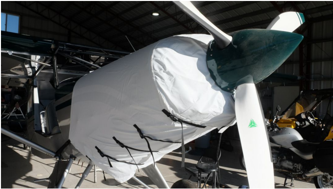
Bearhawk 4 Engine Cover, test fit cover
