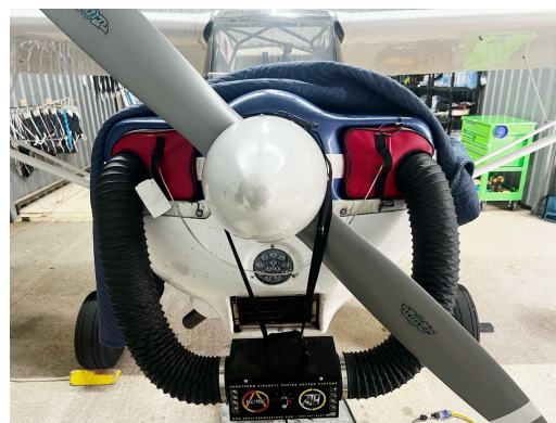
Citabria Engine Inlet Plugs with Aerothem heater hose cutouts.
