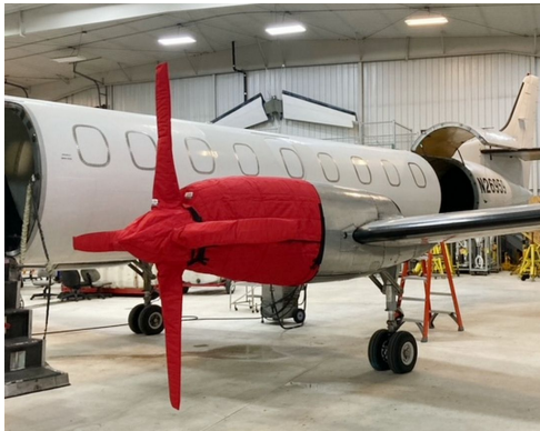
Fairchild Merlin Insulated Engine & Prop Covers
