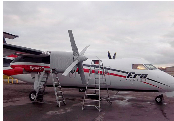
Dash 8 Insulated Engine & Prop Covers
