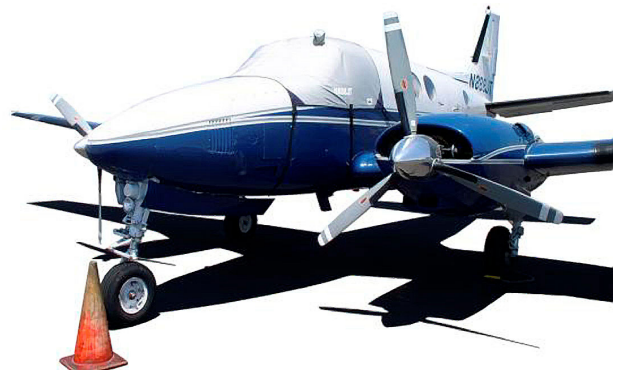
King Air Cockpit Cover, belly-strap type
