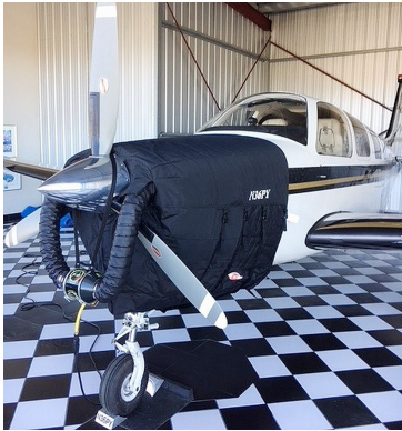
Beech Bonanza 36 Models Insulated Engine Cover
