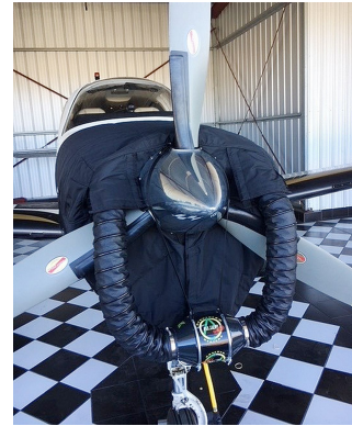
Beech Bonanza 36 Models Insulated Engine Cover
