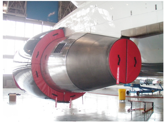
Exhaust Plugs Ship Set, incl. Fan Thrust Reverser and Exhaust Plugs P/N: B767-200
