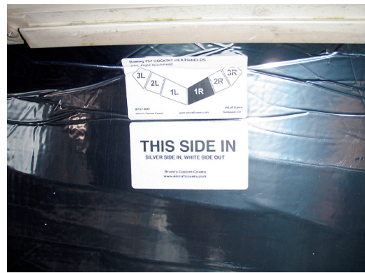
Boeing 757 Cockpit HeatShield set, installation detail
