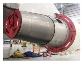
Boeing 747 Bypass Vent & Turbine Exhaust Pugs
