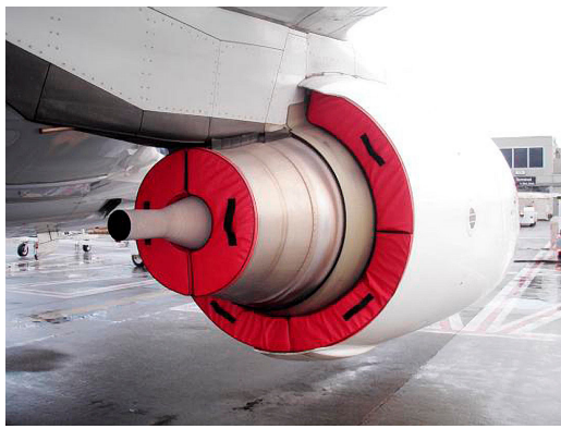
Boeing 737 Bypass and Exhaust Plugs
