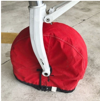
Beech King Air 300 Tire Covers (nose gear)
