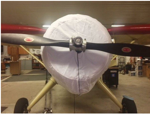
Stinson V77 Insulated Engine Cover, test fit cover
