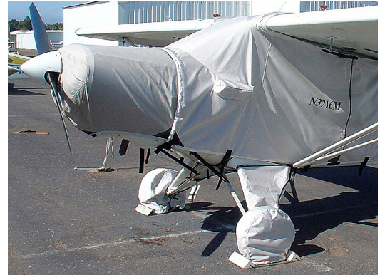
Piper PA-12 Landing Gear Covers
