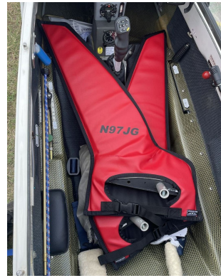
Schempp-Hirth Ventus-2B winglet/wingtip pads
