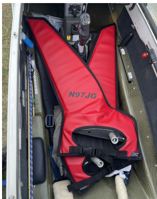
Schempp-Hirth Ventus-2B winglet/wingtip pads
