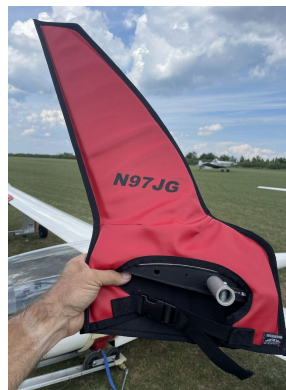
Schempp-Hirth Ventus-2B winglet/wingtip pads
