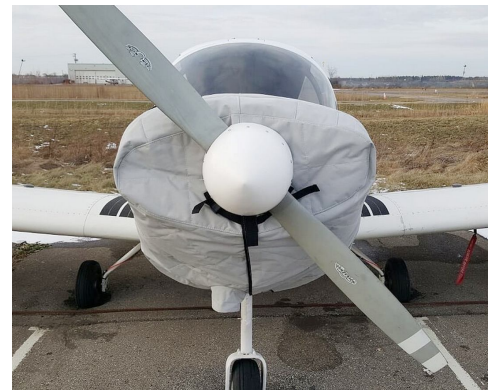
Alarus CH-2000 Insulated Engine Cover
