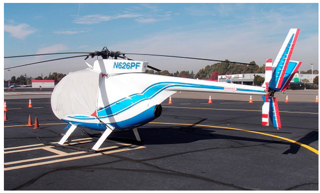
MD500C Bubble Cover with Wire Strike detail
