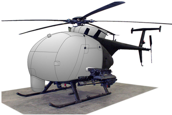
MH-6J Bubble, Flir & Doghouse Covers (illustration)
