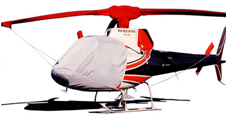
Airbus H-125 & Aerospatiale AS350 Intake/Exhaust Cover, Main Rotor Hub Cover with Weighted Skirt Bubble Cover, Intake/Exhaust, Rotor Mast, Tail Rotor & Main Body Covers
