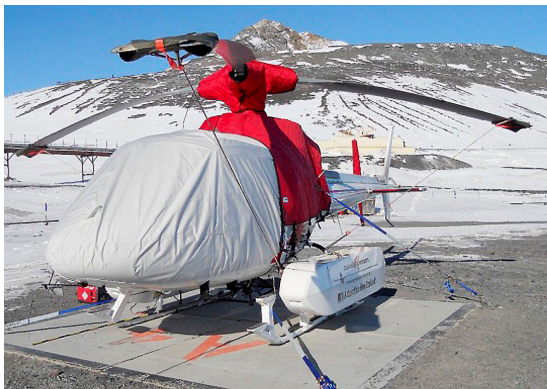
AS355 Bubble Cover w/ Cargo Mirror, Blade Tie-downs, Insulated Engine, Insulated Main Rotor Hub and Insulated Tail Rotor Covers
