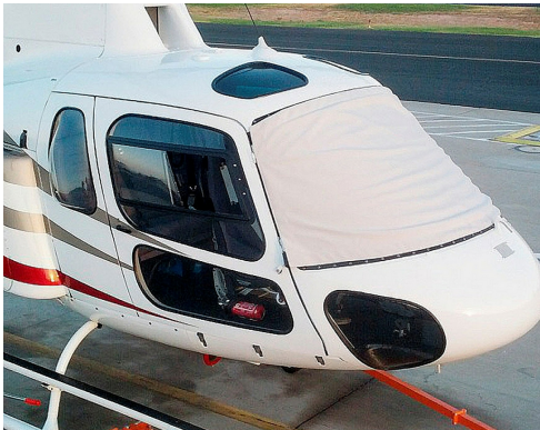
AS350 Windshield Cover, pinches in door jambs
