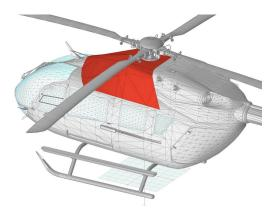
Barrier Inlet Filter Cover, 3D Rendering
