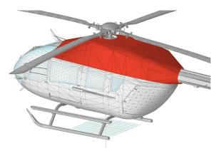
Intake/Exhaust Engine Area Cover, 3D Rendering
