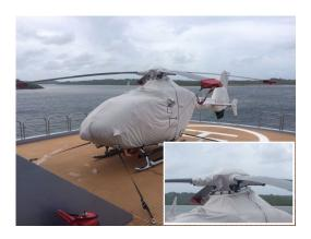
Airbus Helicopter AH135 Main Rotor Hub Cover
