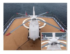
Airbus Helicopter AH135 Main Rotor Hub Cover
