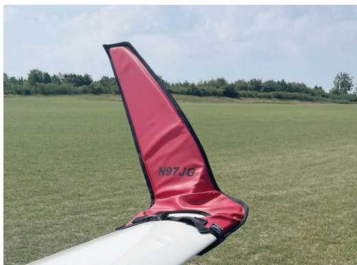
Schempp-Hirth Ventus-2B winglet/wingtip pads
