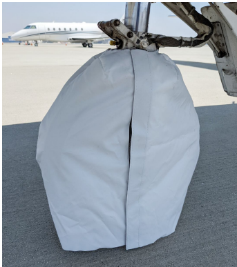
CJ1 Nose Gear Tire Cover, test fit
