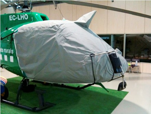
AS350 Bubble Cover with Wire Strike and Cargo Mirror Eurocopter AS350-B3 Bubble Cover w/Wire Strike & Cargo Mirror details.
