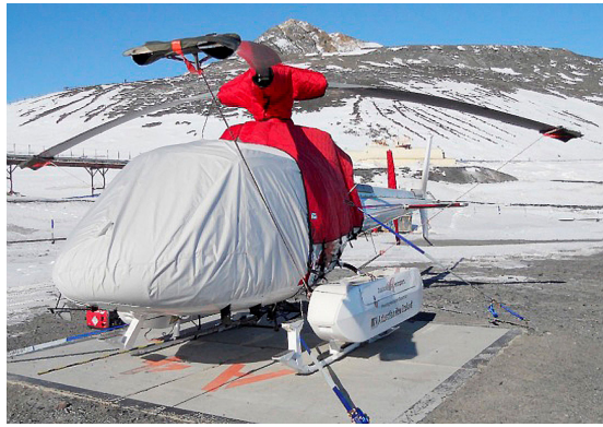
Airbus Helicopter H350 Bubble/Rotor Mast, & Intake Covers AS350 Bubble Cover w/ Cargo Mirror, Blade Tie-downs, Insulated Engine, Insulated Main Rotor Hub and Insulated Tail Rotor Covers
