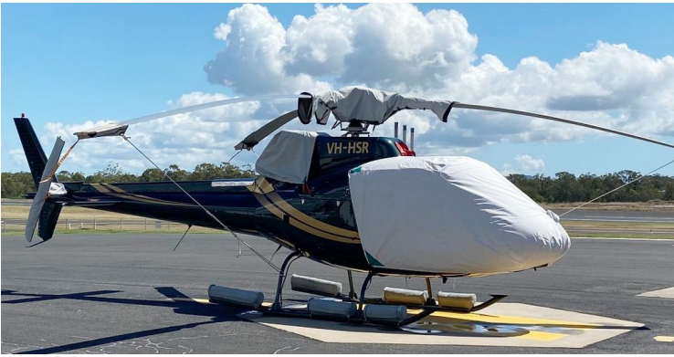
Airbus Helicopter H350 Bubble/Rotor Mast, & Intake Covers AS350 Bubble Cover w/ Cargo Mirror, Blade Tie-downs, Insulated Engine, Insulated Main Rotor Hub and Insulated Tail Rotor Covers
