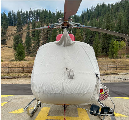
AS350 Bubble Cover with Wire Strike and Cargo Mirror Eurocopter AS350-B3 Bubble Cover w/Wire Strike & Cargo Mirror details.
