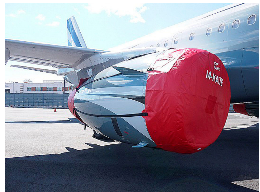
Airbus A319 Intake/Exhaust Covers set, IAE V2500
