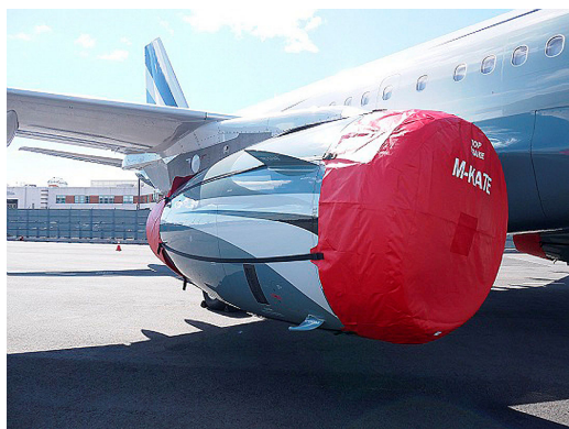
Airbus A319 Intake/Exhaust Covers set, IAE V2500
