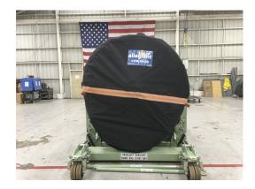
CFM56-5B Off Link Cover, fully enclosed
