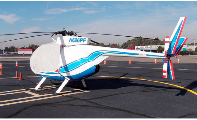
MD500C Bubble Cover with Wire Strike detail
