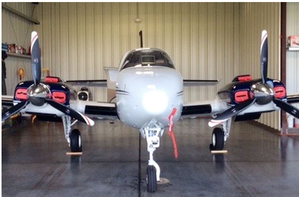
Beech Baron 58 Engine Inlet Plugs, Cowl Top Plugs, Heater Inlet, Pitot Cover
