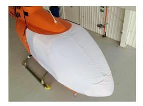
Bell 505 Bubble Cover, test fit cover.
