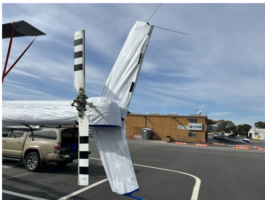
Bell 505 Tailboom & Stabilizer Covers, test fit cover
