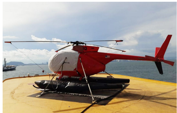
Hughes 500C (369HS) Bubble Cover, Blade Tie-Downs
