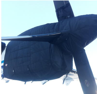
ATR-72-202 Insulated Engine & Prop Hub Covers
