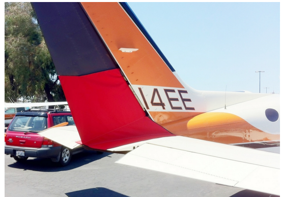
Cessna 414 Rudder Openings Cover (bird barrier)
