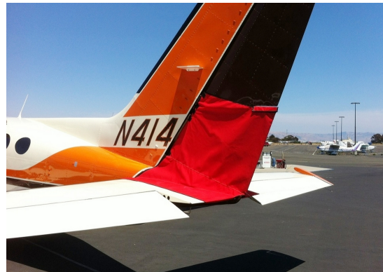
Cessna 414 Rudder Openings Cover (bird barrier)
