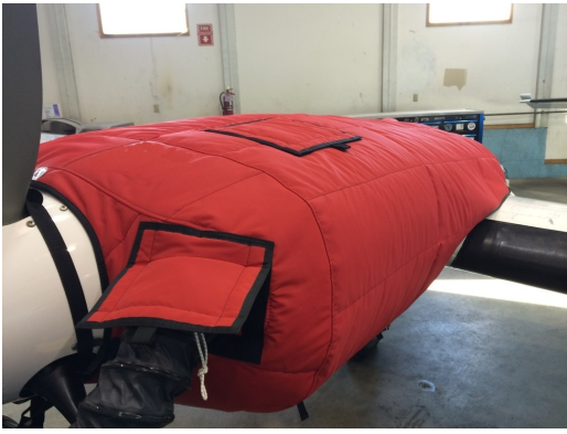
Cessna 402 Insulated Engine Cover with Heater
