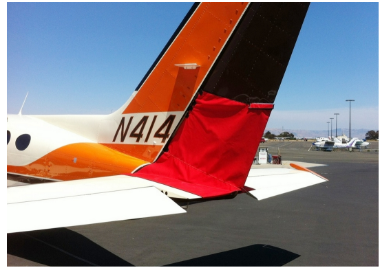
Cessna 414 Rudder Openings Cover (bird barrier)
