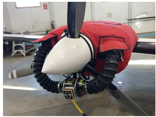
Cessna 402 Insulated Engine Cover with Heater
