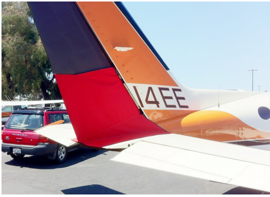
Cessna 414 Rudder Openings Cover (bird barrier)
