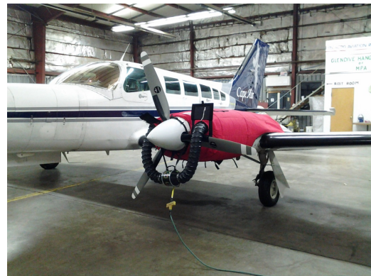
Cessna 402 Insulated Engine Cover with Heater
