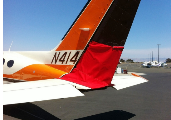
Cessna 414 Rudder Openings Cover (bird barrier)
