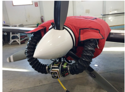
Cessna 402 Insulated Engine Cover with Heater
