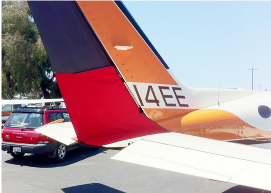
Cessna 414 Rudder Openings Cover (bird barrier)
