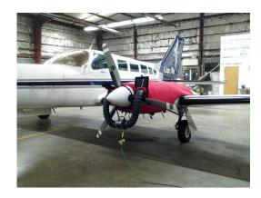
Cessna 402 Insulated Engine Cover with Heater
