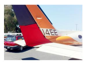
Cessna 414 Rudder Openings Cover (bird barrier)
