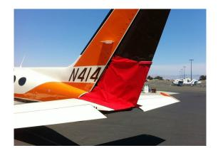
Cessna 414 Rudder Openings Cover (bird barrier)
