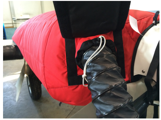
Cessna 402 Insulated Engine Cover with Heater
