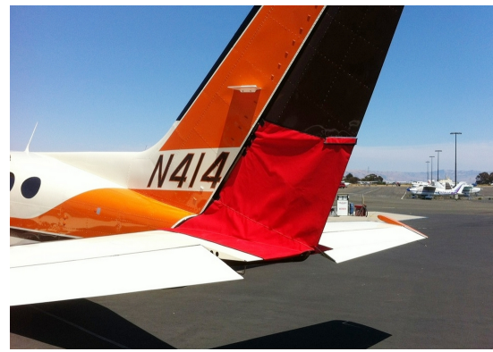
Cessna 414 Rudder Openings Cover (bird barrier)
