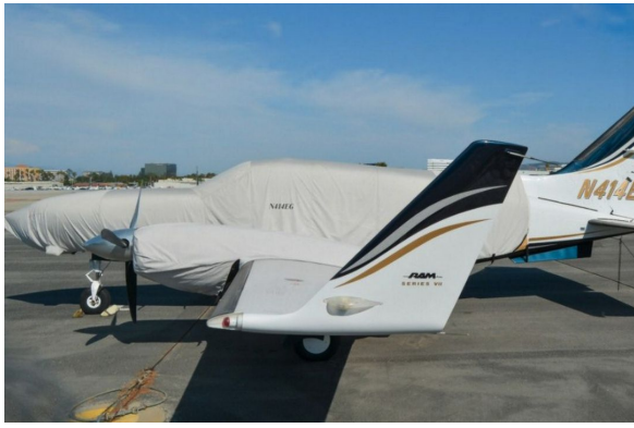
Cessna 414 Extended Canopy/Nose Cover, Engine Covers
