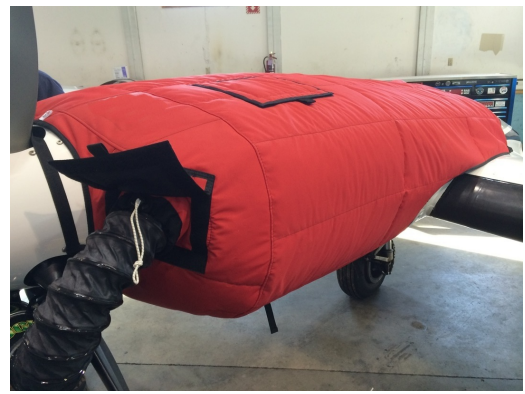
Cessna 402 Insulated Engine Cover with Heater
