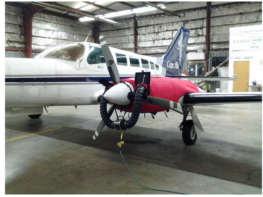
Cessna 402 Insulated Engine Cover with Heater
