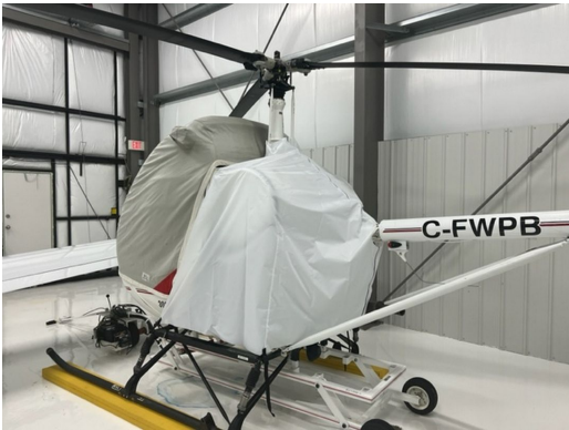
Schweizer 300C Engine Cover, test fit cover
